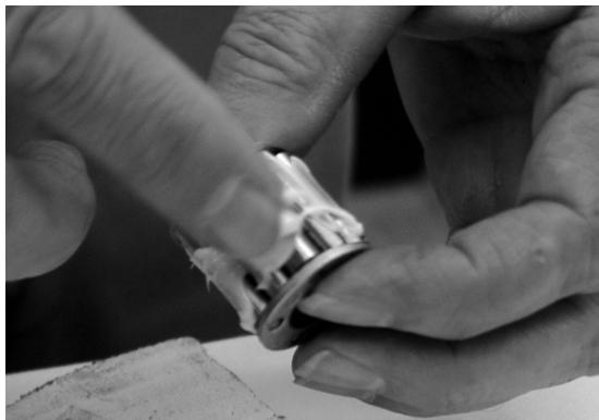
Pack bearing with a water-resistant grease such as white lithium-base or automobile chassis lube. Reassemble bearing and end cap in roller. Spin rollers on shaft to check for free rotation. Reassemble rollers and shafts on carriage. Adjust roller contact until friction between roller and rail prevents roller from turning freely while carriage is stationary.
